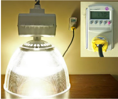
Example Induction High-bay fixture with close-up of wattmeter showing only 170W of power consumption.
