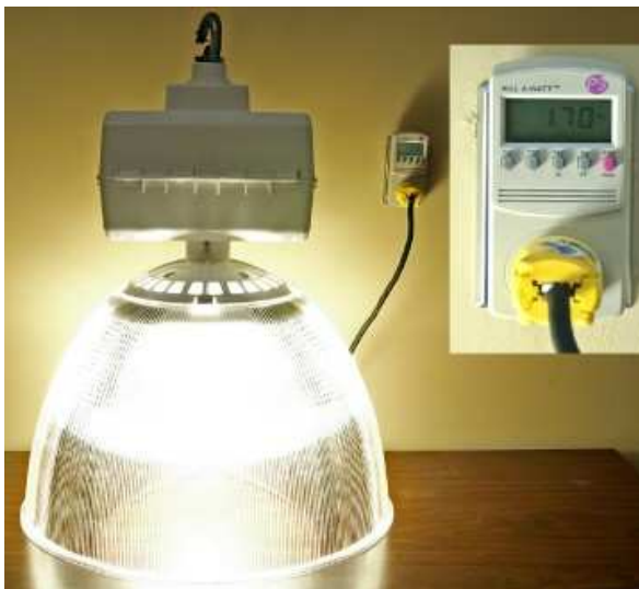
EXAMPLE INDUCTION HIGH-BAY FIXTURE, WHICH CAN REPLACE A 400W METAL HALIDE FIXTURE, WITH CLOSE-UP OF WATTMETER SHOWING ONLY 170W OF ELECTRICAL POWER CONSUMPTION.
